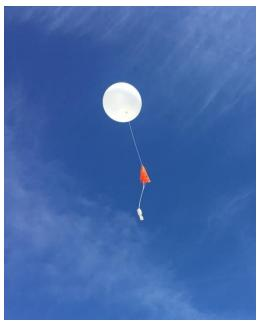
Launching radiosondes upwards
