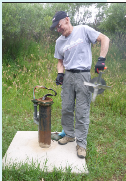
Carefully measuring groundwater level in a well using steel tape method.
